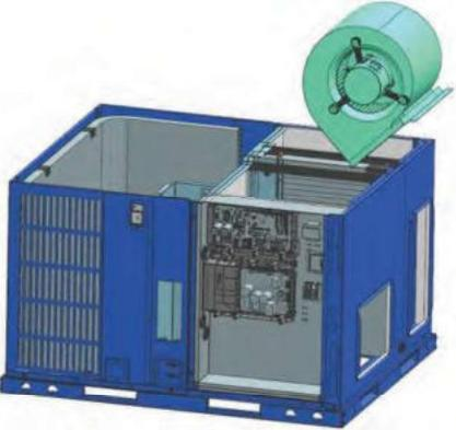
A 3D cutaway diagram of a blue outdoor unit. The top cover is partially removed, and a green indoor fan is shown floating above the unit's interior, indicating its removal. The internal components, including a control board, are visible. | <ol style="list-style-type: none"><li>1. Remove indoor motor terminal;</li><li>2. remove the indoor fan from fixed support.</li></ol> |
