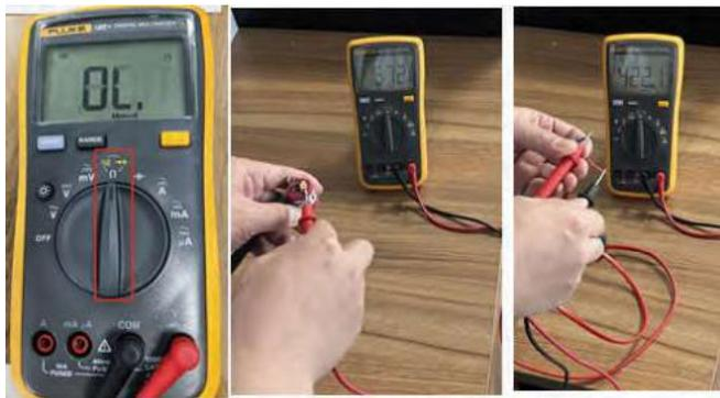
Normally closed switch detection: With no pressure in the pipeline, you can turn a multimeter to the ohm range and connect the red and black probes with a pin (lead) respectively to detect whether the switch is in the "ON" state.
